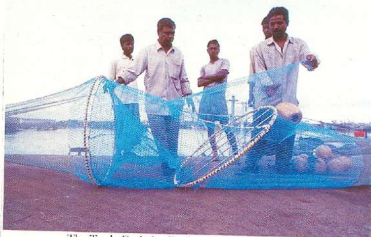
The Turtle Excluder Device (TED) : TED if installed and used properly in the trawl nets can greatly reduce the incidental capture of sea turtles during trawling. The TED designed by CIFT was found to be extremely efficient in excluding turtles from trawl nets
