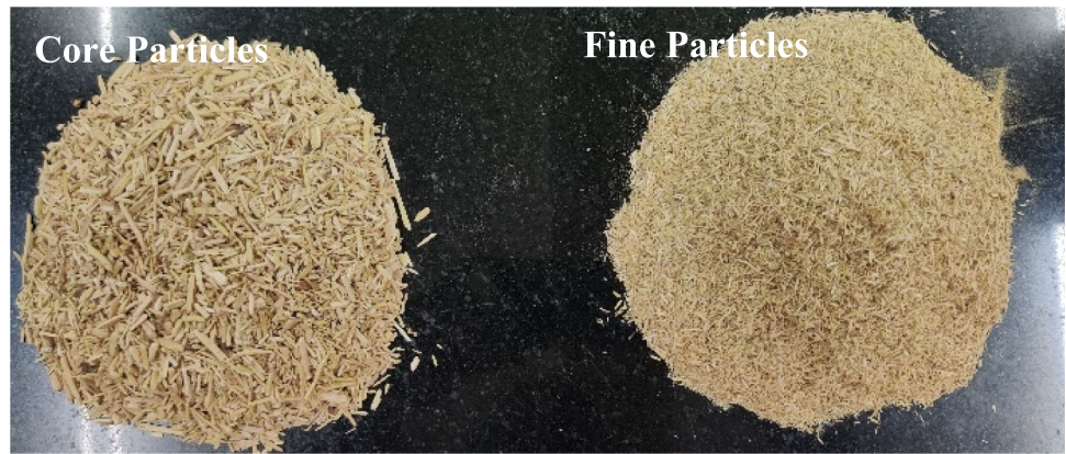
Fig. 2 Segregated core and fine particles based on the size of the particle
