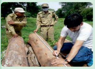
examined and volume was measured. Eccentricity of cross section and frustum of differential length (relative) cones which accounts for tapering nature of timber logs were duly and practically accounted for, during the volume calculation. Following three equations were used for calculating the volume:
