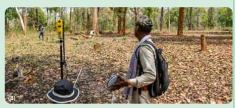
(A) Measurement of tree diameter at different height segments of Bridelia retusa at Dhamtari forest division using Basal Area Finder (BAF) Scope (B) Measurement of tree diameter at different height segments of Adina cordifolia at Bastar forest division using Basal Area Finder (BAF) Scope
