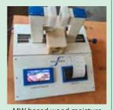
MW based wood moisture measurement system
