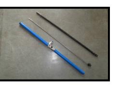
Fig 3. Increment borer and its parts
